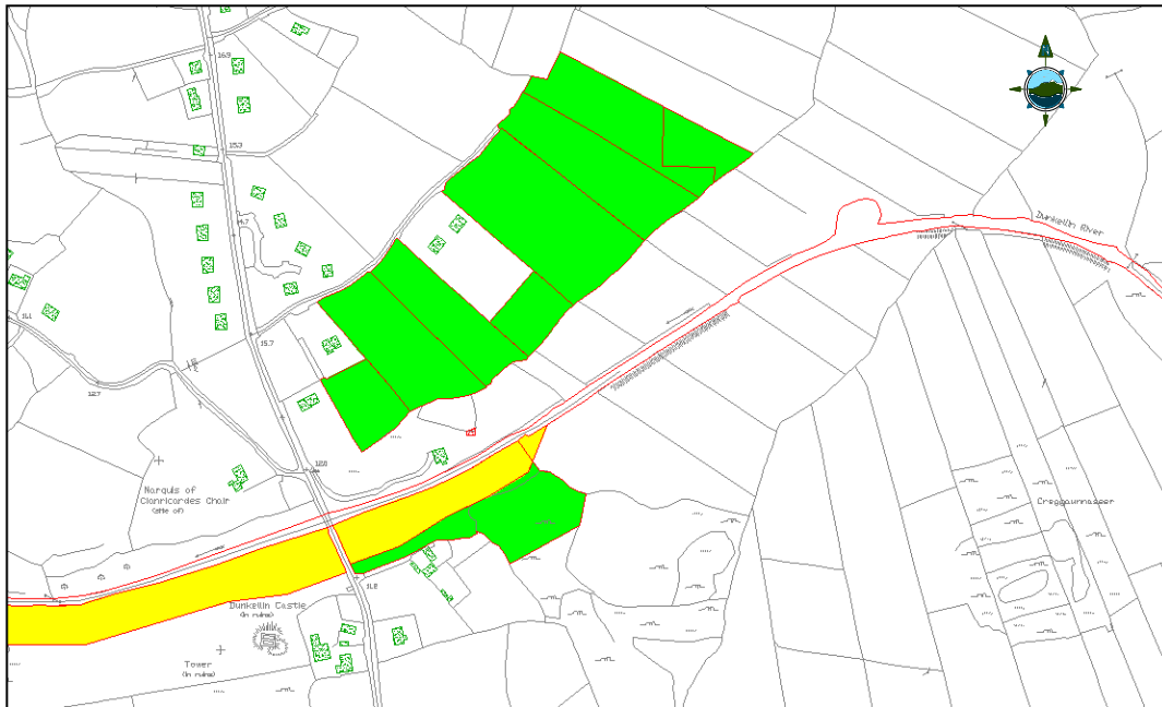
Figure 6-5 – Approximate Location of Lands required for deposition of excavated material (green) upstream of the Dunkellin Bridge (yellow areas indicate extent of channel works)
